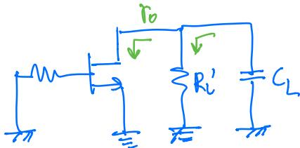
$$R_3 = R'_\text{out} // R_o = R'_\text{out}$$
